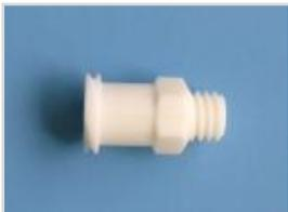
10.32 UNF male thread / Luer female connector. These connectors are used to connect syringes to the following 6.2 mm, 11 mm and 16 mm i.d. columns.
