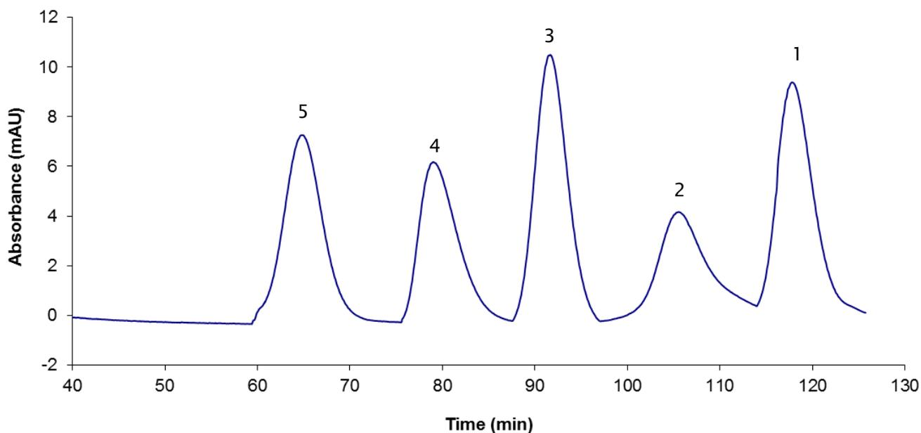
**Figure 2:** Separation of test substances on a ProteoSEC 16/600 3-70 HR gel filtration column. Flowrate: 1 ml/min; sample loading: 0.5 ml; mobile phase: PBS (phosphate buffered saline); Model proteins 1: Vit B-12 (M<sub>r</sub> 1,200); 2: Aprotinin (M<sub>r</sub> 6,500); 3: Cytochrome c (M<sub>r</sub> 12,300); 4: β-Lactoglobulin (M<sub>r</sub> 35,000); 5: BSA (M<sub>r</sub> 67,000).
