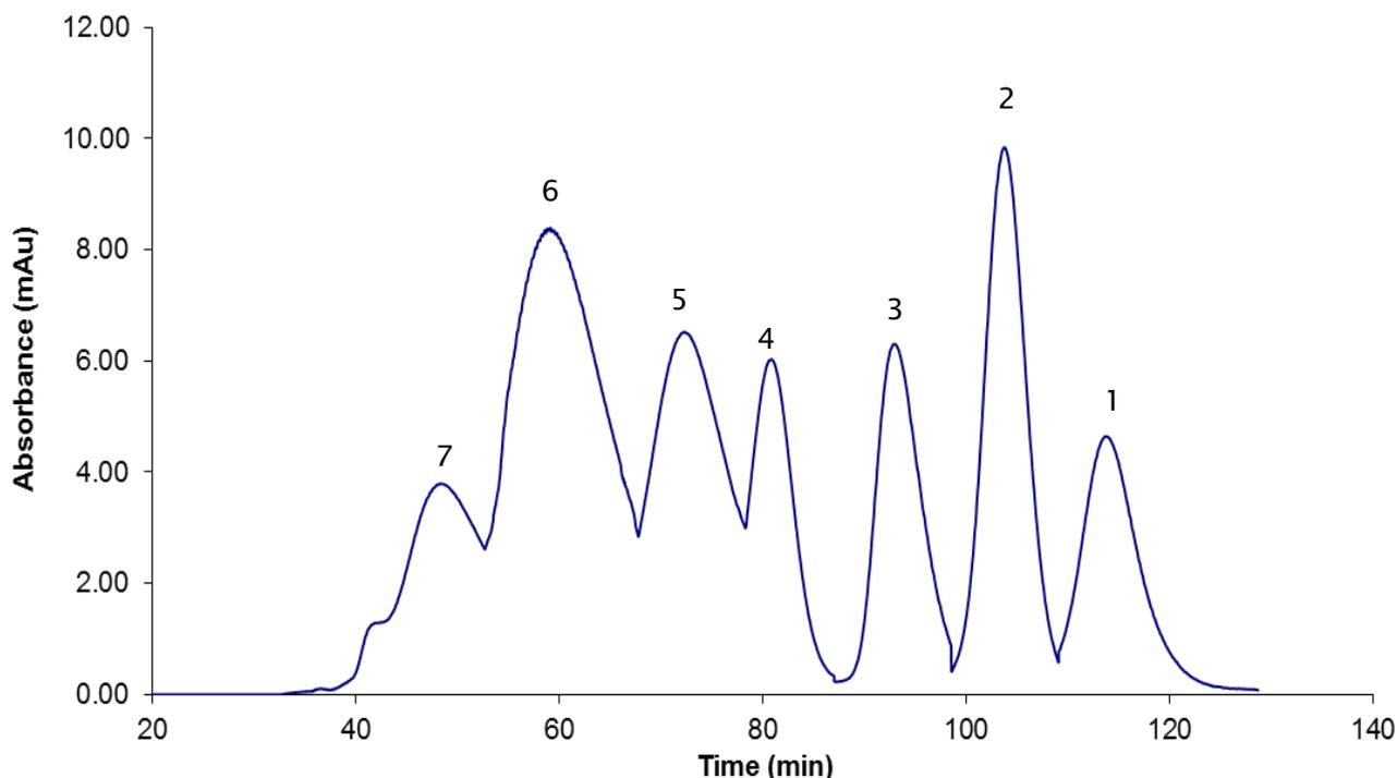
**Figure 1:** Separation of test substances on a ProteoSEC 16/600 6-600 HR Dynamic gel filtration column. Flowrate: 1 ml/min; sample loading 0.5 ml; mobile phase: PBS (phosphate buffered saline); Model proteins 1: Aprotinin (M<sub>r</sub> 6,500); 2: Cytochrome c (M<sub>r</sub> 12,300); 3: β-Lactoglobulin (M<sub>r</sub> 35,000); 4: BSA (M<sub>r</sub> 67,000); 5: γ-Globulin IgG (M<sub>r</sub> 158,000); 6: Apoferritin (M<sub>r</sub> 440,000); 7: Thyroglobulin (M<sub>r</sub> 669,000)
